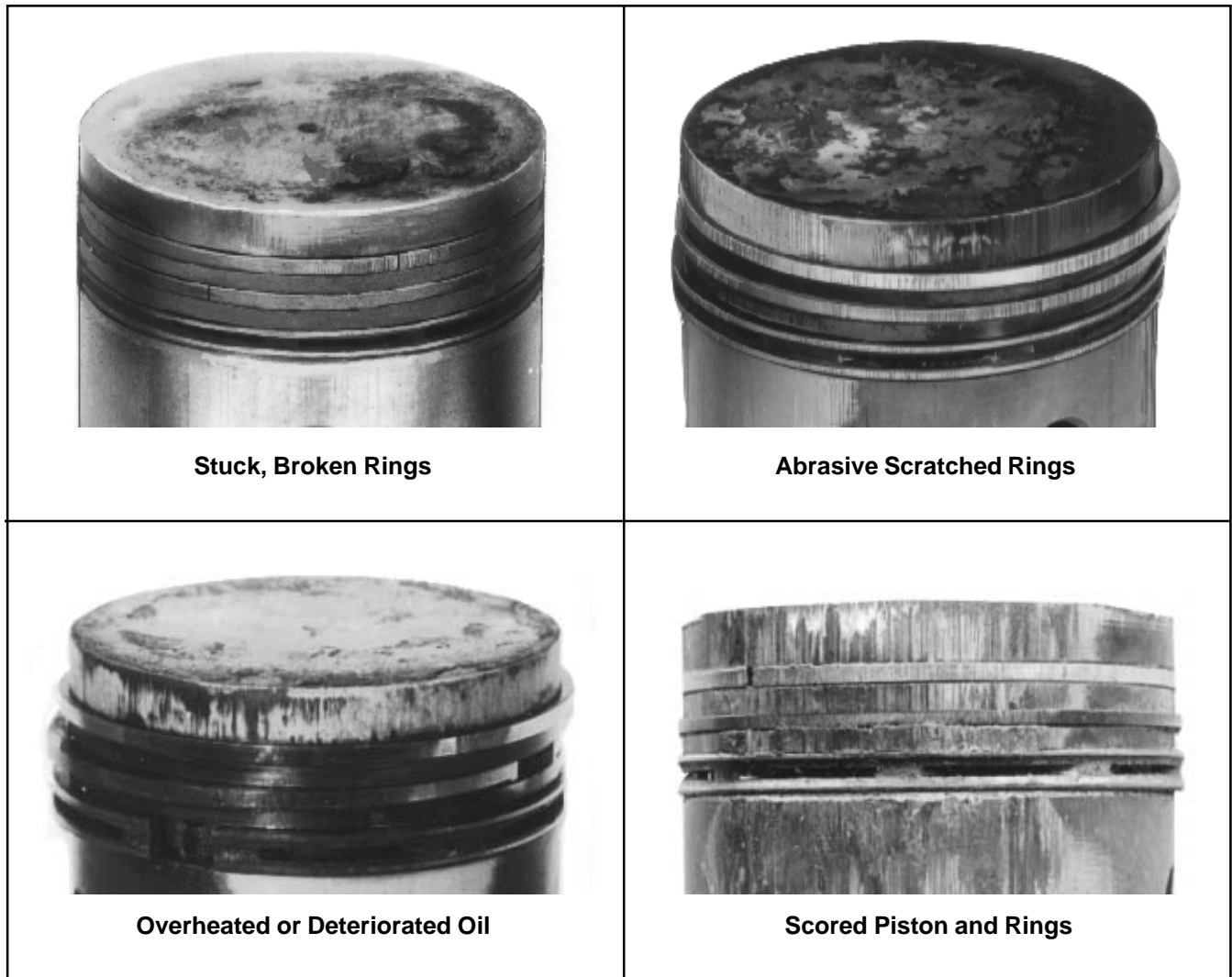
Figure 10-8. Common Types of Piston Damage.
